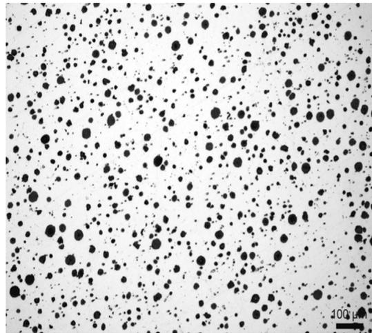
**Fig. 5** Ductile iron with spheroidal graphite. The graphite content of the ductile iron is almost the same as that of cast iron. The spheroidal shape is due to the manufacturing process which makes it stronger in tensile strength and better fracture toughness as compared to the cast iron
