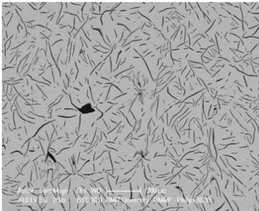
**Fig. 4** Flaky graphite microstructure of cast iron pipe. Cast iron pipes have higher percentage of carbon as compared to other ferrous metals. The flaky graphite is due to the manufacturing process which makes it lower in tensile and fracture toughness properties as compared to the other ferrous metals
