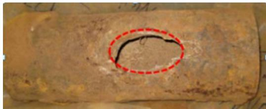
**Fig. 8** Old exhumed cast iron pipe with the blown section. This pipe section was received from City West Water, Melbourne, Australia, for the investigation of carrying out research in RMIT, University, Australia. Blowout failure is developed by internal water pressure. In this situation, pitting corrosion causes pipe to be thin until water pressure blows out remaining
