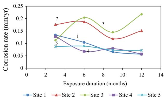
**Fig. 15** Relationship between corrosion rate and exposure duration for  $3 \times 70$  steel. Initially, corrosion rate for all sites is high except for site 3. With the increase in exposure duration, the corrosion rate is decreasing due to development of stable oxide layer. The irregularity in corrosion behaviour at sites 2 and 3 for an exposure duration of 12 months can be due to the ingress of chloride, which deteriorates stable oxide layer. Modified after Song et al. (2017)
