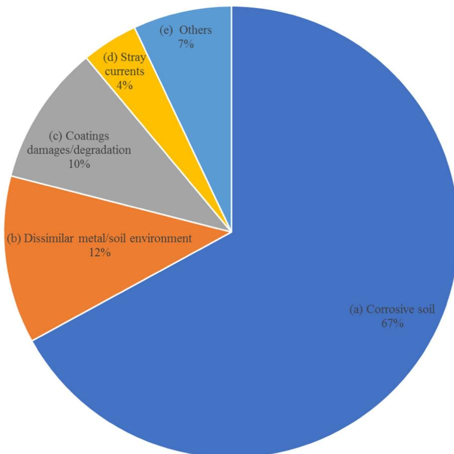
**Fig. 2** Key factors affecting external corrosion of buried pipes. Some of these factors are dependent on each other. Soil resistivity has a direct relationship with moisture content and chloride concentration. As moisture contents and chloride concentration increase, soil resistivity decreases. Aeration of soil can be changed by the rain and the bacterial activity. pH of the soil is affected by acid rain and acid-producing bacteria
